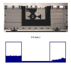
Fig.9 Comparison of water behavior at 0.5 sec. (above: tank model test, below: MPS method)
