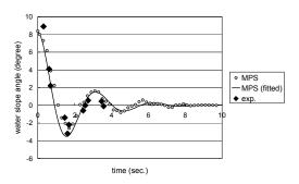
Fig.10 Comparison of damping curve with  $D_t\!=\!7.5mm$  and  $W_t\!=\!30mm$
