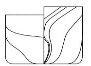
Fig.7 Body plan of the post-Panamax containership
