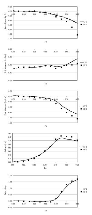
Fig.4 Comparison of hydrodynamic force and attitude in heeled condition between CFD and EFD
