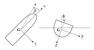
Fig.3 Coordinate systems of the measurement
