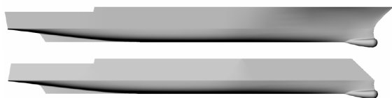
Fig. 1: ONR Topside Series Hull Forms- ONRFL (top) and ONRTH (bottom).
