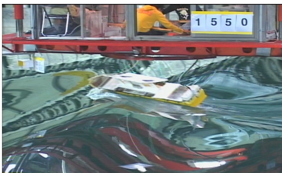
Fig. 6: Photograph of Large Roll Motion in Quartering Sea (GM=1.2m, \lambda=1.5L_{pp} , Vs=25kts, \chi=15deg , H/\lambda=1/18 )
