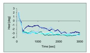
Figure 25 Roll versus time, Hs=4m, D2
