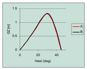
Figure 3 Comparison of righting levers
