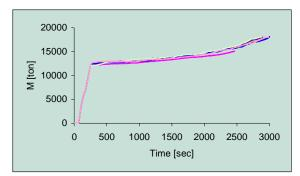
Figure 26 Mass versus time, Hs=4m, D1
