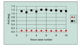
Figure 16 RMS heel for Hs=2m, damage D1
