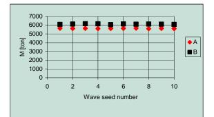
Figure 22 Floodwater mass for Hs=2m, D2
