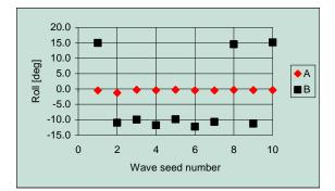
Figure 13 Mean heel for Hs=4m, damage D1
