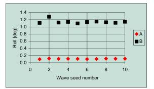
Figure 18 RMS heel for Hs=2m, damage D2
