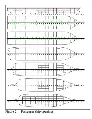
Two damage positions were chosen: with centre at frame 100 (D1) and with centre at frame 180 (D2). The latter position is near mid ship. Both damage positions were at the starboard side of the ship. The damage length extended along two compartments. Discharge coefficients were to be determined by the participants.
