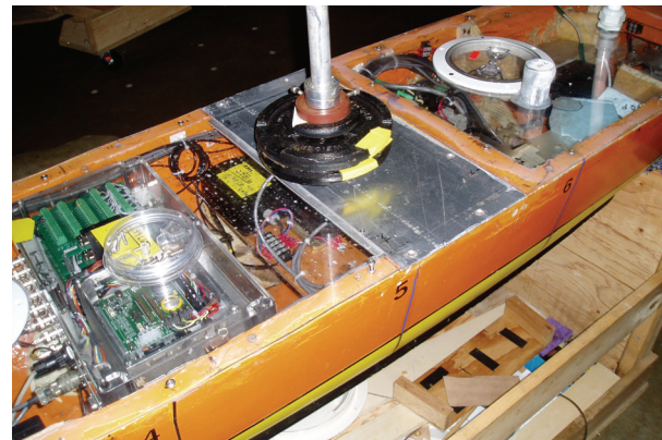
Figure 3. Midship OBC, GM Pole, and instruments.
