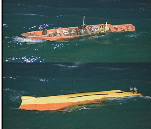
Figure 1. View of Model 5514 During Capsize Testing In MASK Basin.
