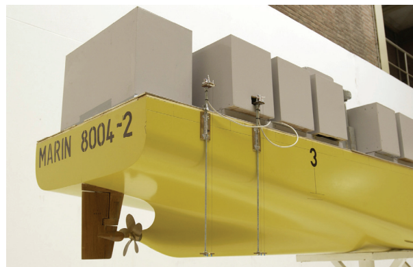
Fig. 3—Stern-Quartering View of MARIN Model 8004-2 Showing Rudder and Propeller (MARIN, 2009).
