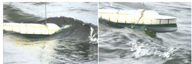
Fig. 4. Trawler hulls balanced by the lack of running trim in calm water, and this dynamic stabilization is not affected on a large stormy waves, where the motion of the wave energy goes mainly in heave, with no direct impact on the propulsive quality and stability on the storm course
