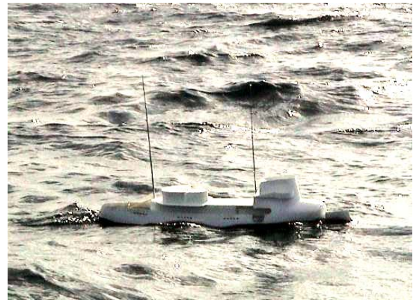
Fig.7. Rounded ship hull and lower deck of the vessel reduces the intensity of all types of storm rolling on deep water
