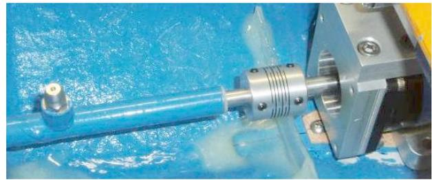
Fig. 4 – Connection of motor and propeller shafts
