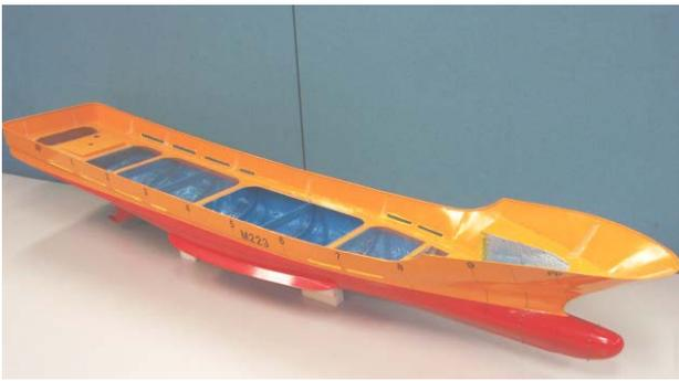
**Fig. 1 – Ship model for free-running tests**
