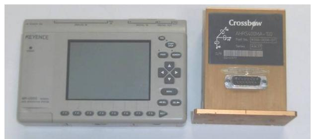
Fig. 7 –Data logger and 6DOF inertial sensor
