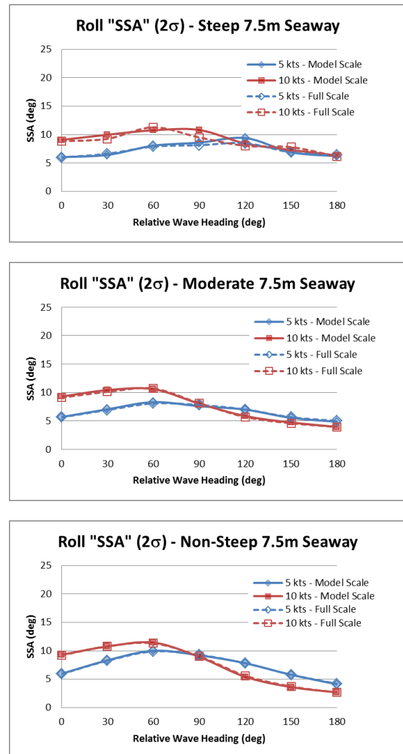
Fig. 5: “Non-rare” statistics of roll motion at H_s = 7.5 m at 5 kt (blue) and 10 kt (red) for model scale (solid) and full scale (dashed), shown at three modal periods: top) T_m = 10 s; middle) T_m = 14 s; bottom) T_m = 17 s
