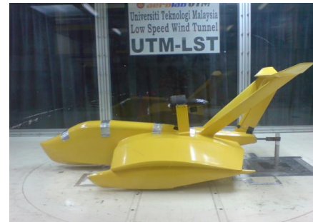
Fig. 3 - Wind tunnel test for WIG craft model [12]
