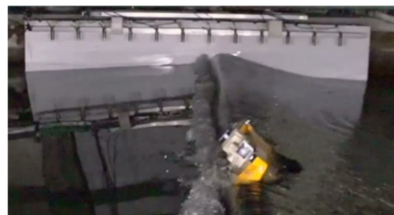
Figure 1.1: The experiment for the breaking wave hitting
