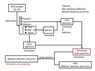
Figure 1: Basic concept of the proposed system.
