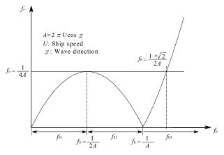
Figure 2: Relationship between encounter wave frequencies and absolute wave frequencies.
