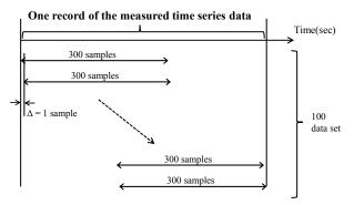
Figure 3: Schematic diagram concerning the contraction of the data set.
