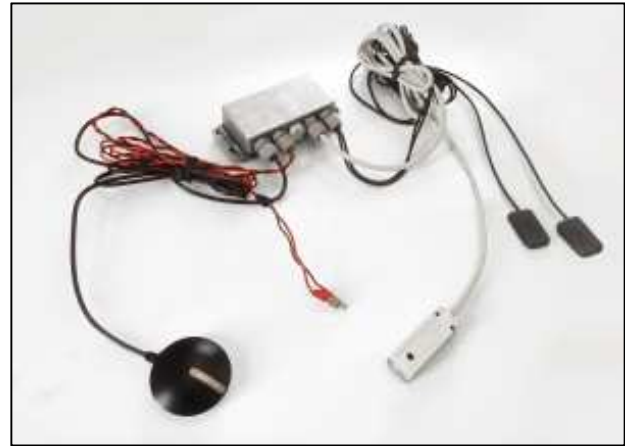
Figure 2: Vibration measurement system.
