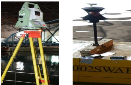
Figure 2: The theodolite and the prism attached on the model ship
