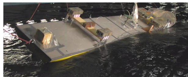
Figure 8: Still from the experiment in regular head waves at maximum roll angle: \zeta_a = 3.0 m, \omega = 0.50 rad/s. V_s = 5.5 kn.
