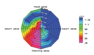
Figure 8 Two polar plots for limiting capsizing wave height for a wave length of 172m. Left: GM=0.8m Right: GM=1.9m
