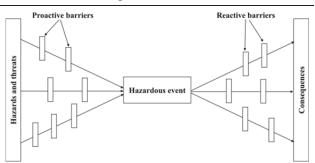
Figure 3: Simplified bowtie diagram [5]
