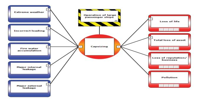
Figure 5: High level bowtie diagram, only showing threats and consequences.
