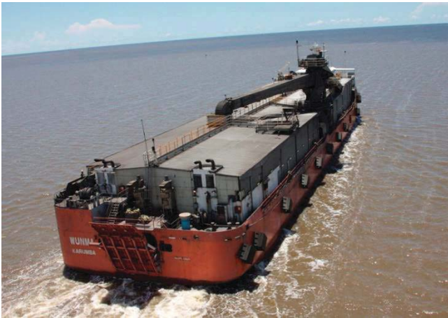
Figure 5 - MV Wunma, with a well deck configuration
