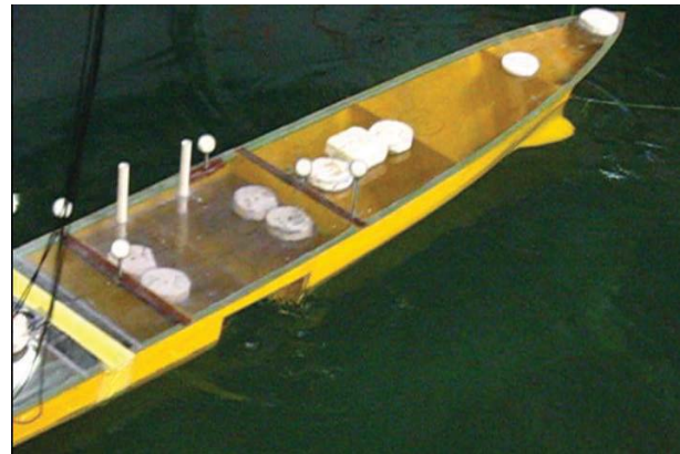
Figure 2 Damage opening of DTMB 5415
