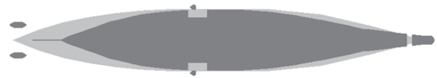
Figure 11 Parallel waterplanes for d=6.00 m (light grey) and d_L=3.33 m (dark grey).
