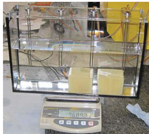
Figure 2 The level sensors during calibration
