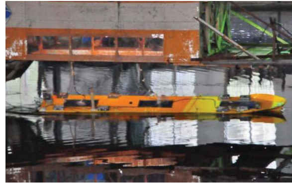
Fig.6 The ship model in free decay test
