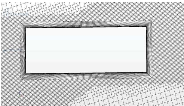
Figure 5 - Refined mesh around the body
