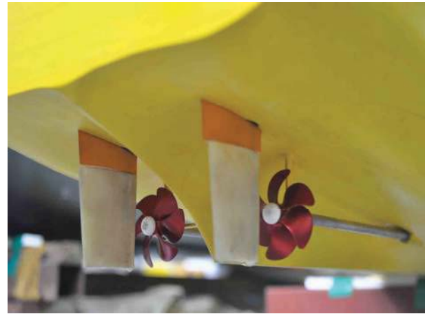
Figure 5 Fully appended stern of the test model.
