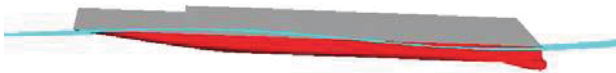
Figure 12: LAMP simulation of ONR Topsides tumblehome hull in irregular following seas (Spyrou et al. 2012)
