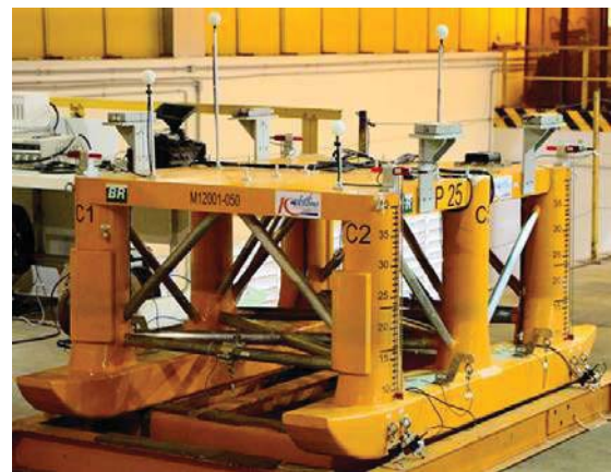
Figure 2 – SS Model in Laboceano Basin
