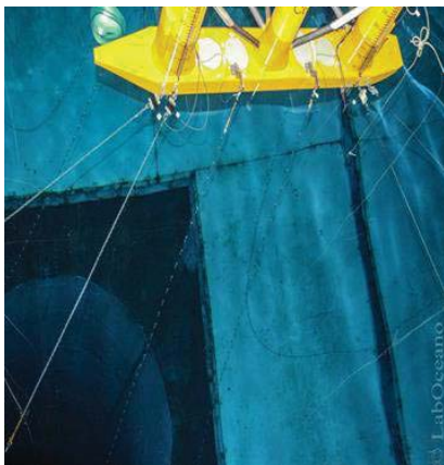
Figure 3 – Mooring and Risers Model
