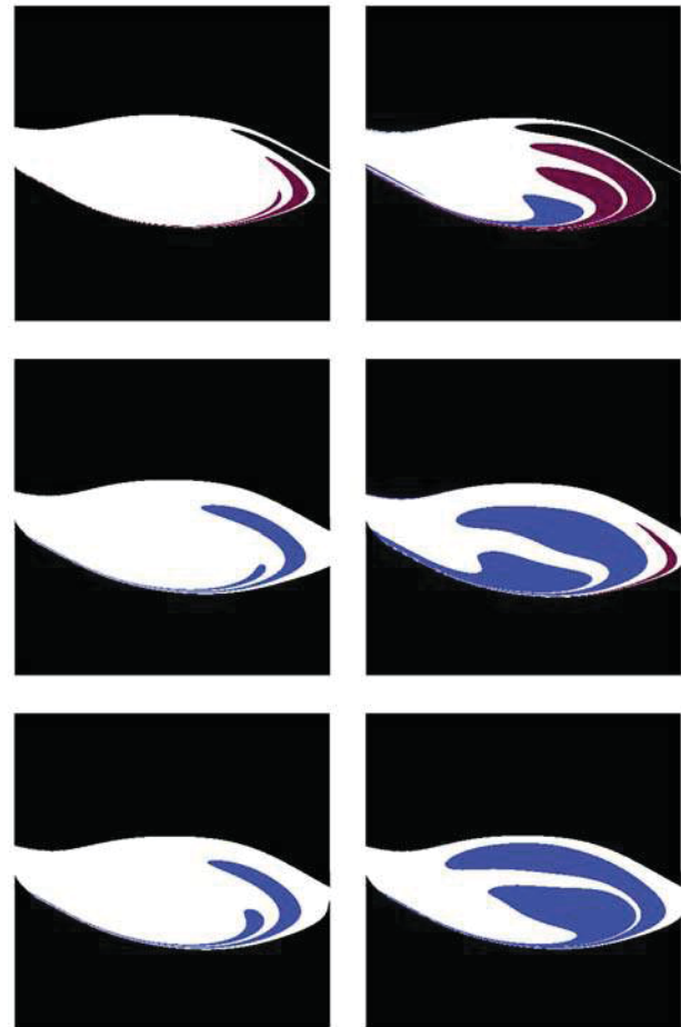
Figure 10: Transient basin erosion. Left column: 10% integrity loss; right column: 40% integrity loss; from top to bottom: Cases 01, 02, 03.
