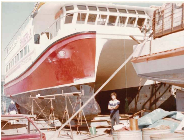
Figure 1 - Shangri La 20m Catamaran, hull centrelines toe out, asymmetric hulls with bulbs. Strathclyde Ph D. Student Apostolis Tsanticos standing in photo.
