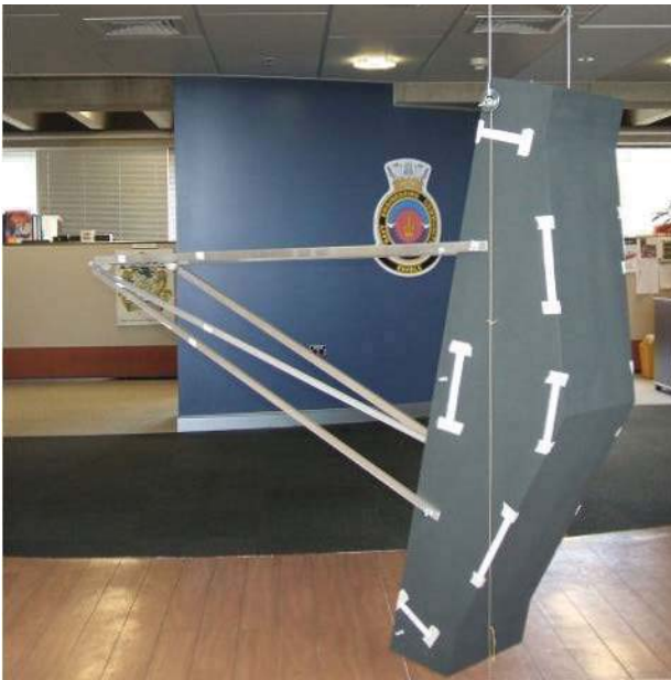
Figure 4 Establishing KG by suspension
