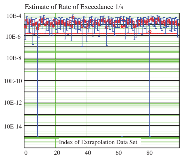
Figure 6 Confidence interval overlap of true value for lateral acceleration at 45 deg heading at 0.2g comparison level using logarithm CI
