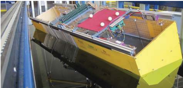
Figure 1 The inclined model in the test basin after flooding
