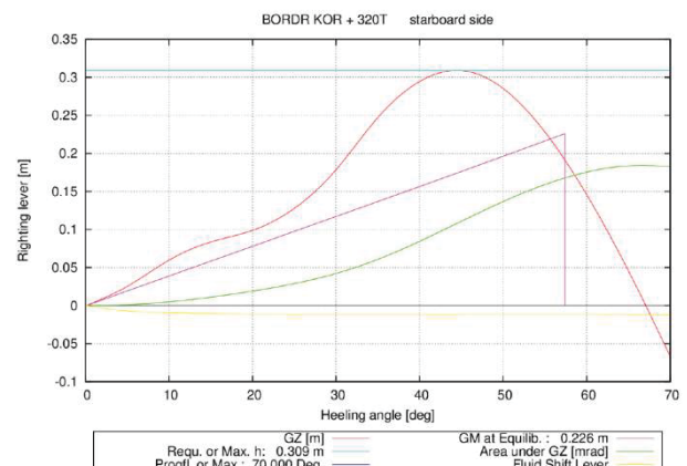
Figure 9 Lever arm curve at departure time in Riga with corrected centre of gravity and cargo load
