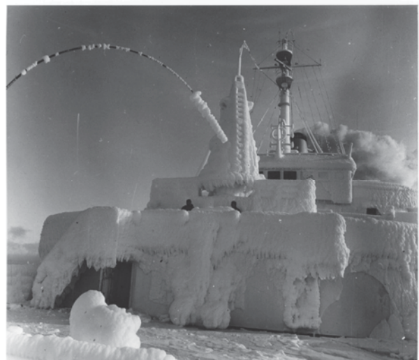
Fig.1. Severe icing on m/s Stefan Batory in North Atlantic. (Courtesy of Captain H.Majek)
