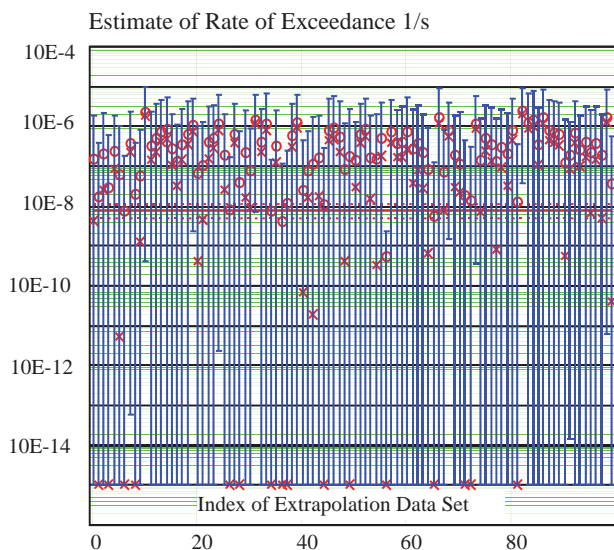
Figure 4 Confidence interval overlap of true value for pitch at 45 deg heading at 11.5 deg comparison level using logarithm CI (98%)
