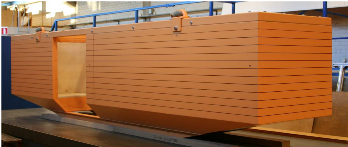
Figure 1.2 The bow and stern sections, connected with the backbone structure
