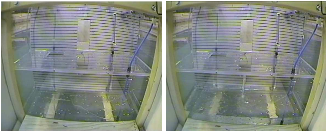
Figure 4.63 Test05 – air pocket in DB1 is visible (left) before the flooding from R21 to R11 (right)
