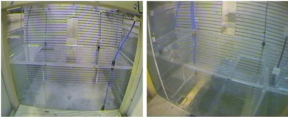
Figure 4.62 Test05 – highly turbulent flooding in DB1 (left) and the start of flooding to DB2 (right)
