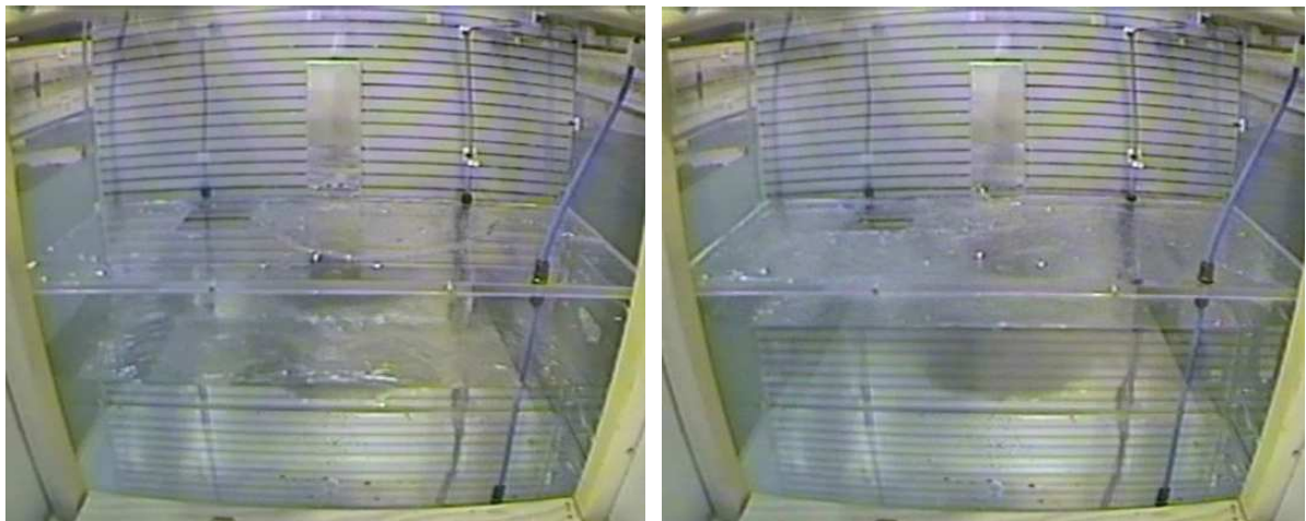
Figure 4.30 Test03 – down-flooding from R12 to R11 (left: R12 is flooded through the open WT-door; right: the down-flooding starts)
