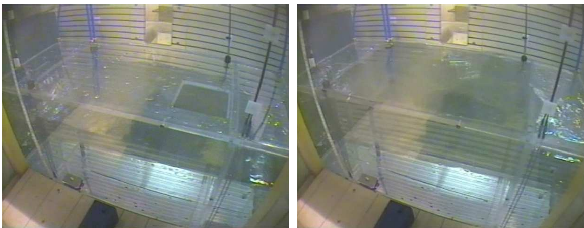
Figure 4.80 Test06 – the free surfaces are parallel when the damage opening is fully submerged (left) and the side compartment R21P is not yet filled when the up-flooding to R22 starts (right)
