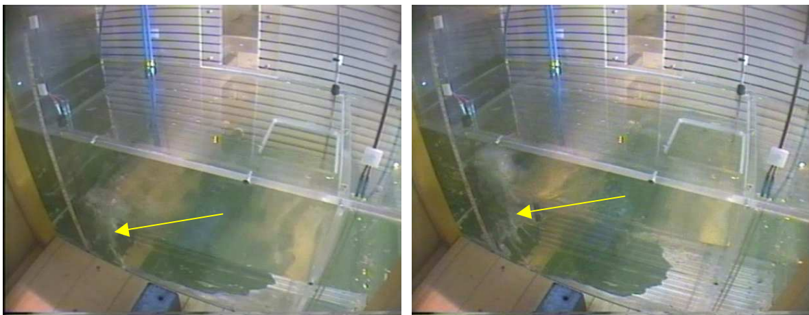
Figure 4.3 Test01 – video captures from the air bubbling (pointed by the arrows)
