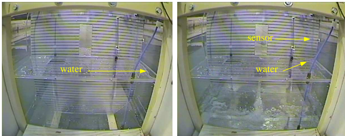
Figure 4.46 Test04 – small initial volume of water in the room R12 (left) is collected around the water height sensor (right) as the model trims
