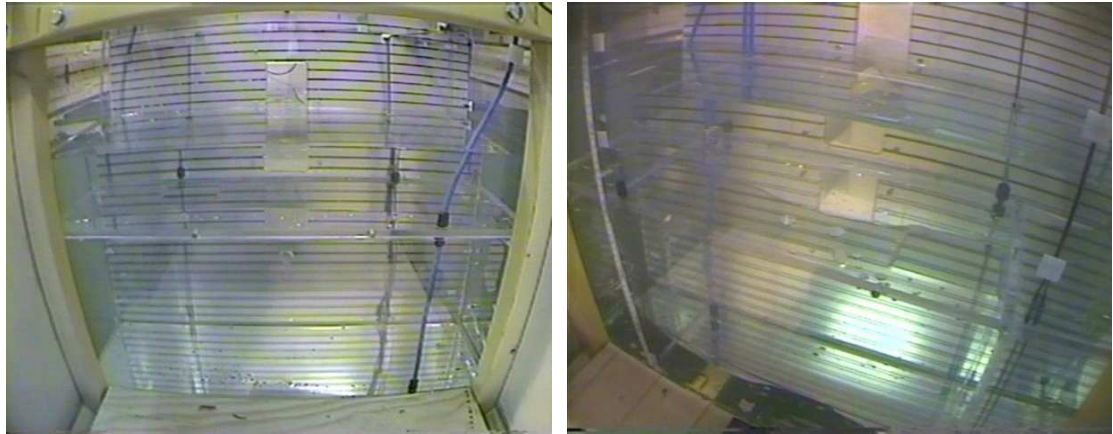
Figure 4.15 Test02 – video captures from the equilibrium condition (on left the aft compartment and on right the forward compartment)
