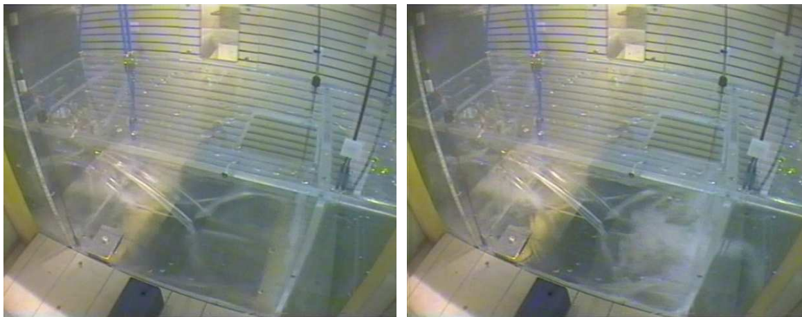
Figure 4.79 Test06 – video captures from the early stages of the flooding; the plate that closes the manhole to the double bottom is clearly visible
