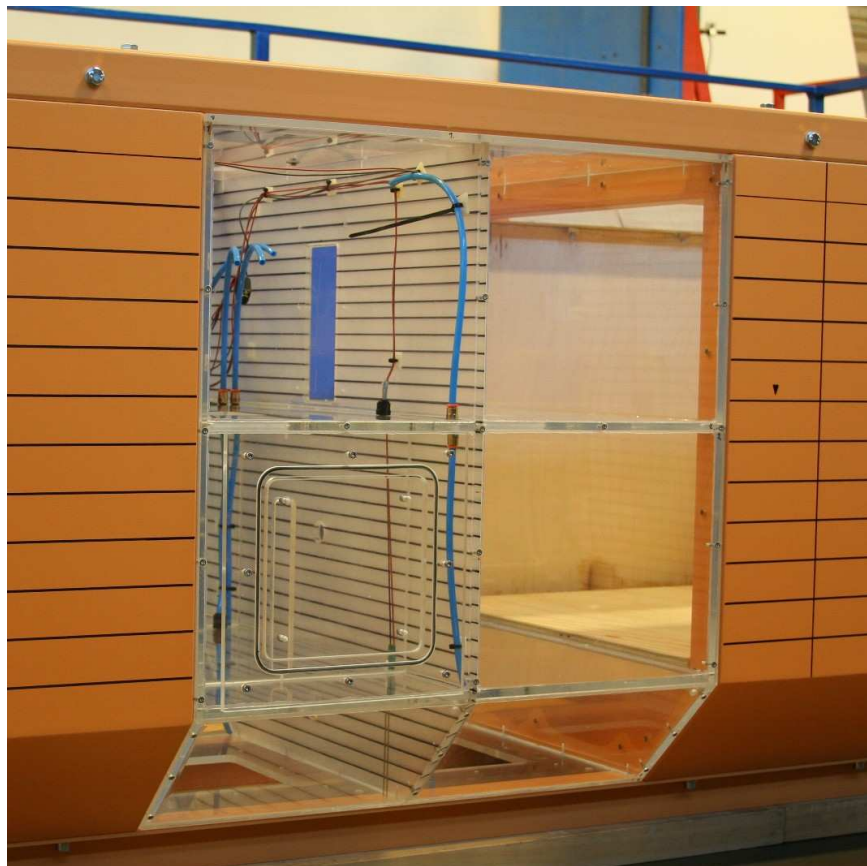
Figure 1.8 The mid-section installed in the model
