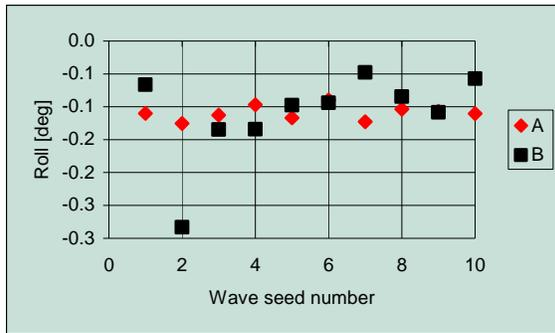
Figure 14 Mean heel for Hs=2m, damage D2
