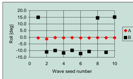
Figure 13 Mean heel for  $H_s=4m$ , damage D1
