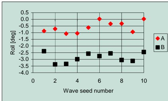
Figure 15 Mean heel for Hs=4m, damage D2
