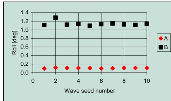
Figure 18 RMS heel for Hs=2m, damage D2
