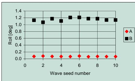
Figure 16 RMS heel for Hs=2m, damage D1
