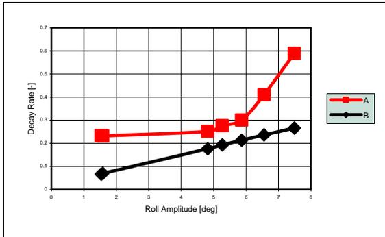
Figure 5 Roll decay rate versus roll amplitude
