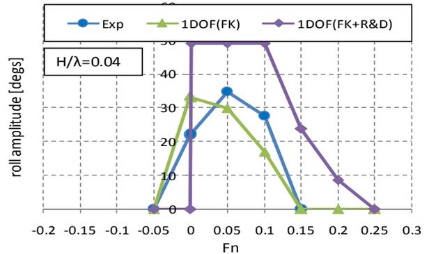
Figure 7: Comparisons of parametric roll between experiments and simulations, under the condition of  $\lambda/L_{pp}=1.0$ ,  $\chi=0^\circ$  and  $180^\circ$ .
