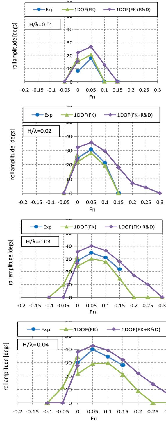
**Figure 5: Comparisons of parametric roll between experiments and simulations, under the condition of  $\lambda/L_{pp}=1.0$ ,  $\chi=0^\circ$  and  $180^\circ$ .**
