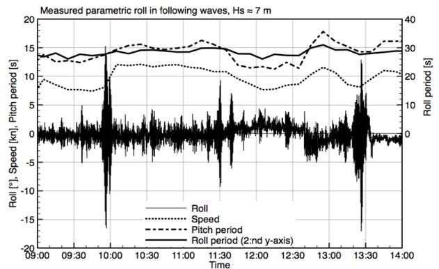
**Figure 8: Sequence with the highest roll amplitudes during the studied 16-month period combined with 10 min average data for speed, pitch period and roll period. The periods have been plotted with different scales to better illustrate the excitation of large amplitudes when there is a perfect 2:1 relation between roll periods and pitch periods.**
