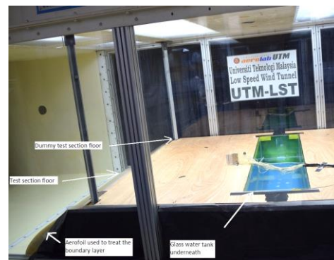
Figure 8: Arrangement in the test section.
