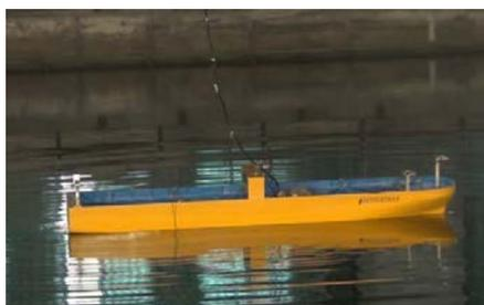
Figure 4: Free roll decay tests of the pure car carrier.
