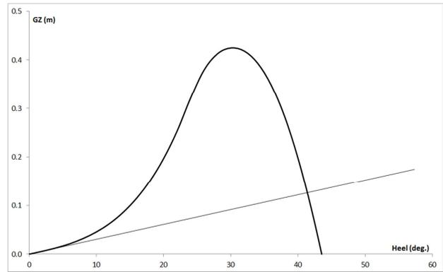
Figure 16: GZ curve of the tanker.
