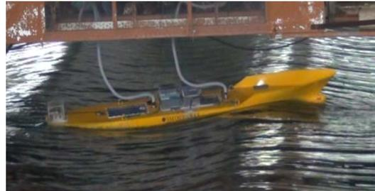
**Figure 3: The passenger ship model in the free running experiment.**
