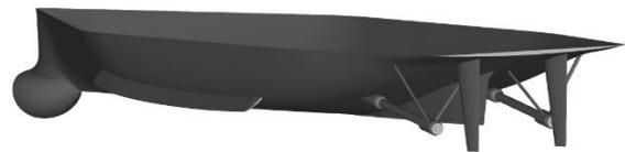
**Figure 2: Underwater geometry of ONRTH.**
