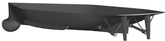
Figure 2 Underwater geometry of ONRTH.
