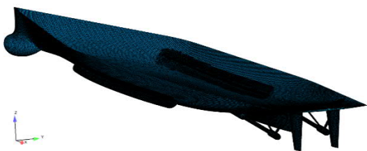
Figure 3 Quadri-lateral surface grid elements on the ONRTH hull.
