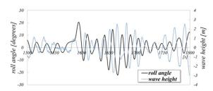
Figure 1: Numerical simulation of the RoPax ship with the roll restoring variation.
