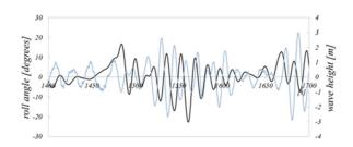
Figure 2: Numerical simulation of the RoPax ship without the roll restoring variation.
