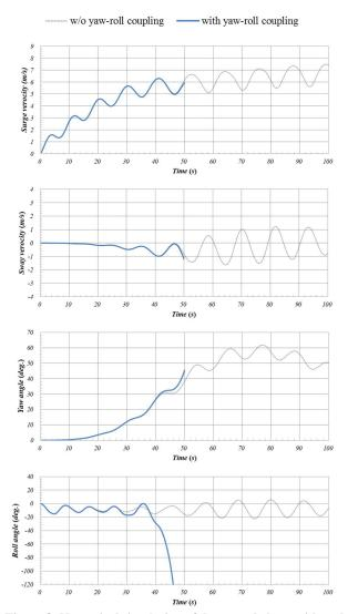
Figure 8: Numerical simulation of the torpedo boat with and without yaw-roll coupling. Here the wave steepness of 0.06, the wavelength to ship length ratio of 1.0, the Froude number of 0.26 and the heading angle of 50 degrees from the wave direction.
