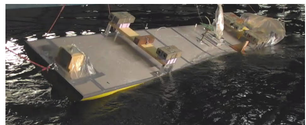
Figure 8: Still from the experiment in regular head waves at maximum roll angle: \zeta_a = 3.0 \text{ m} , \omega = 0.50 \text{ rad/s} . Vs = 5.5 kn.
