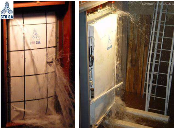
Figure 2: Door tests in full scale at CTO's laboratory in Gdansk, Poland
