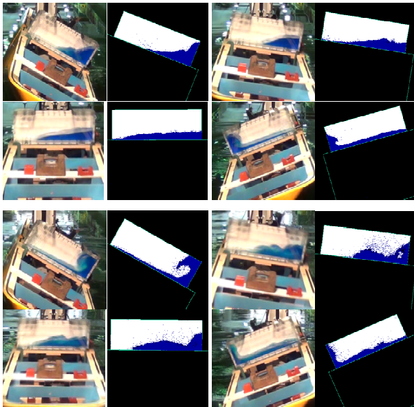
Figure 7: Comparisons of the water deformation between the experiment and the MPS simulation with \phi_a=30\text{deg.} for the rectangle tank (above: T_\phi=3.25\text{sec.} , below: T_\phi=1.75\text{sec.} )
