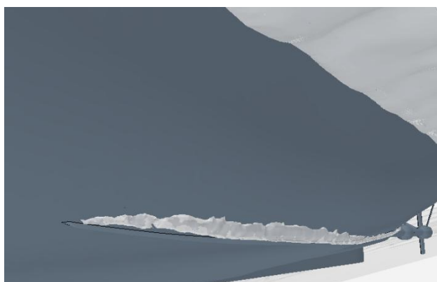
Figure 11: Entrapped air in the simulation due to emerging and re-entering bilge keel - T = 14.6 [s], \varphi_A = 35 [°], Fn = 0.13 -
