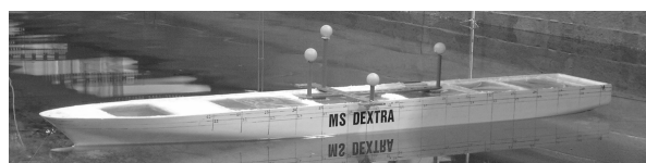
Figure 2: The Ro-Ro model in the towing tank with the Qualisys markers in place.
