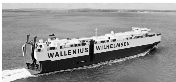
Figure 1: The Panamax Pure Car and Truck Carrier that serves as case vessel in this paper.
