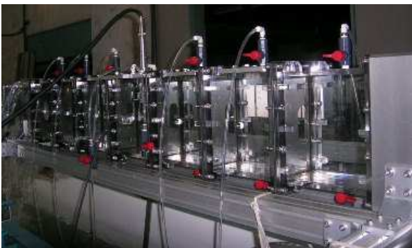
Figure 4: Photo of the six cross-duct modules. (The 1:10 scale model).
