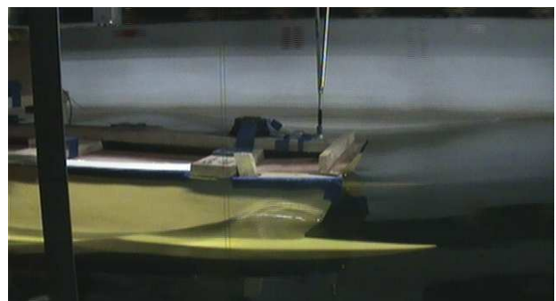
Figure 9: Seakeeping test in following sea, conducted in towing tank.
