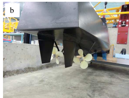
Figure 2: Bow and stern of the ONRTH model: (a) bow; (b) stern.
