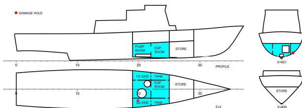
Figure 5: Damage scenario for the full-scale flooding case.
