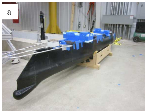
Figure 2: Bow and stern of the ONRTH model: (a) bow; (b) stern.
