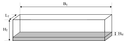
Figure 2: Definition of parameters of the rectangle tank.
