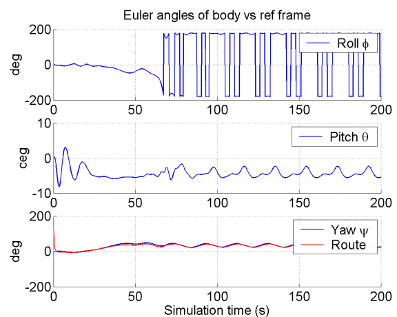
Figure 7: Euler angles obtained with the simulator for the first wave conditions.
