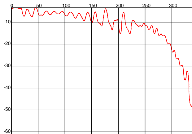
Figure 11: Heeling angle vs time [sec] for 0.1 sq.m. cardeck downflooding opening area each
