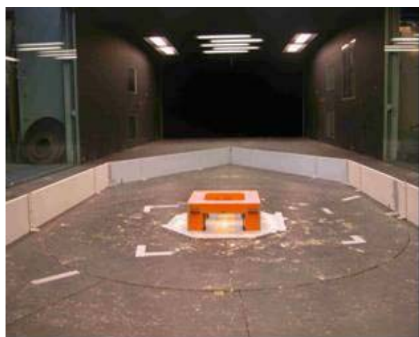
Figure 2 Underwater part in the wind tunnel
