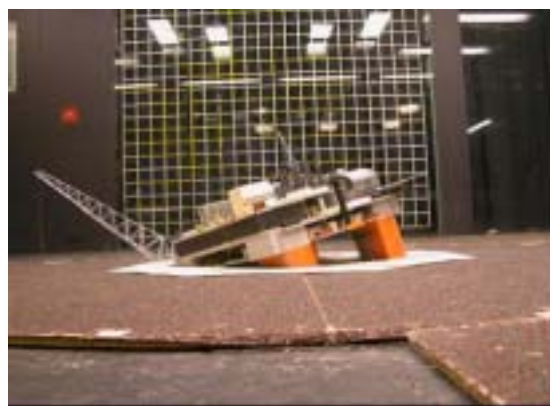
Figure 14 Tunnel Test – Heeled Platform 15 degrees
