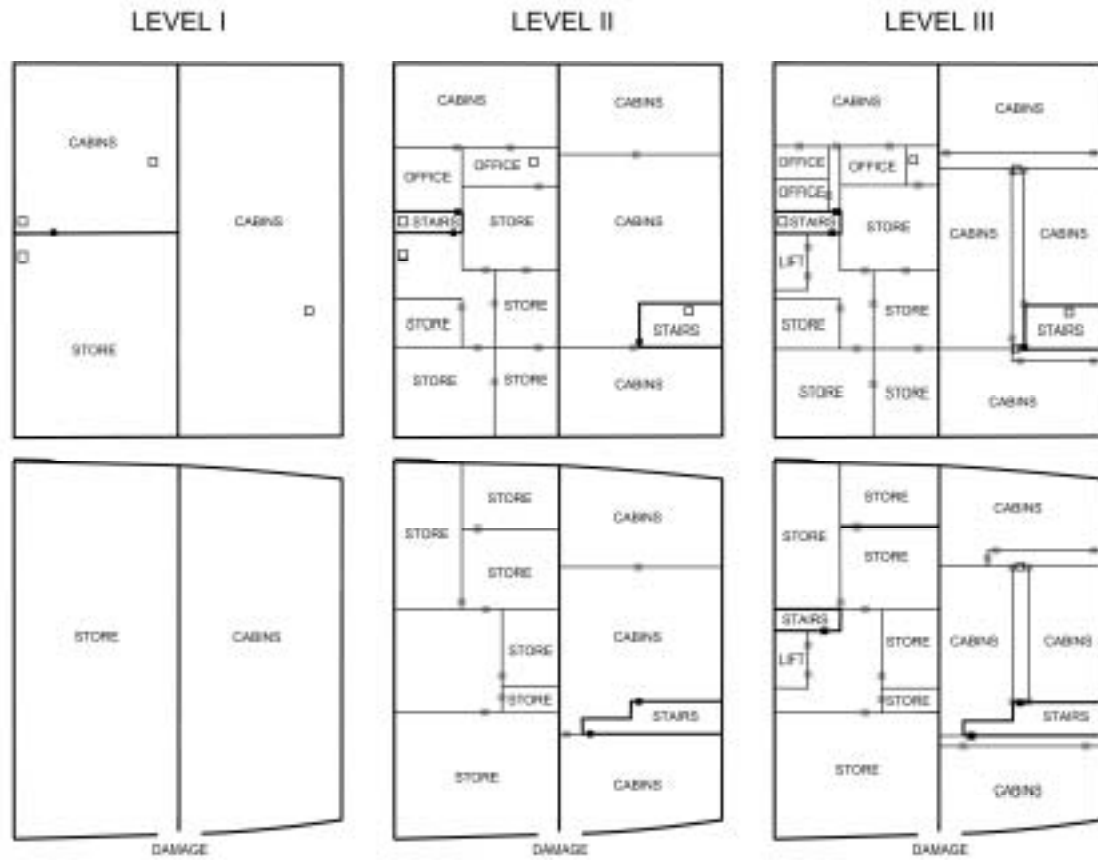
Figure 15 Tested levels of internal modelling; the grey squares mark B-class joiner doors, the black squares mark A-class fire doors and blank squares are connections that are initially open
