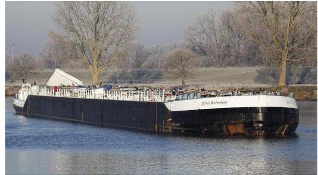
**Figure 4: Tanker, just fallen from weir.**
