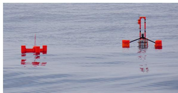
Figure 3.4: The Mini-buoy (Left) and the Ultra-Small-Directional-Wave-Buoy (Right)
