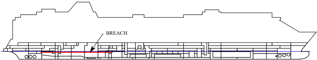
Figure 2: Small breach extending to several compartments
