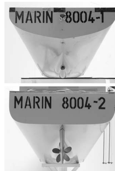
Figure 4 Original C11 (upper) and Pram type (lower) aft ship
