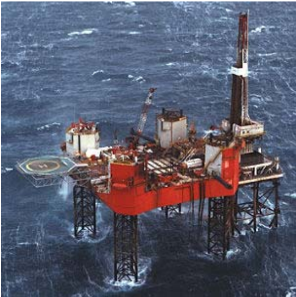
Figure 2 A four leg Jack-up drilling unit in operation
