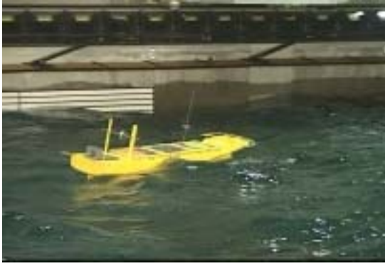
Figure 2 A photograph of free running model experiment in short-crested head waves
