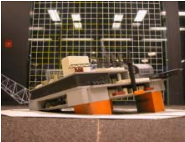
Figure 8 – Tunnel test model at 10 degrees.
