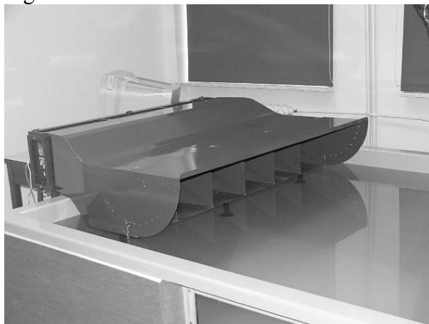
Figure 10. The stand bed for ship's dynamic stability simulation.
