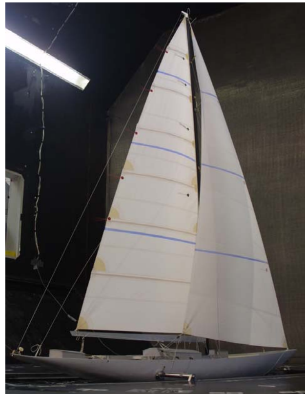
Figure 6. Model used for maximum heeling moment tests.
