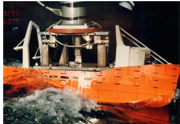
Figure 2. Fully captive model tests in waves (Grochowalski, 1989).
